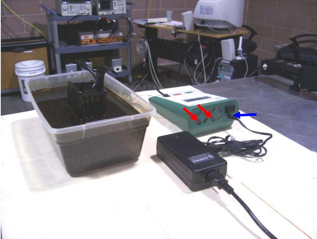
Figure A3. Electrostatic Discharge Test Points.
