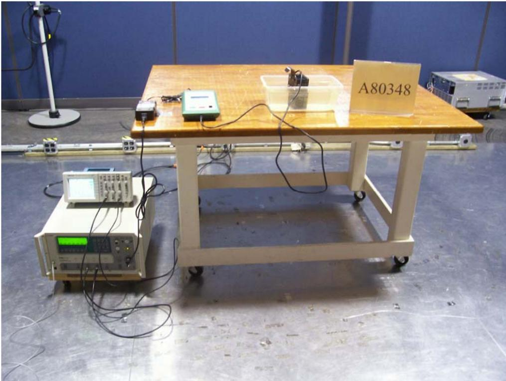
Figure F1. Voltage Dips and Interrupts Test Setup.
