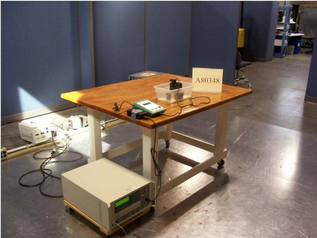
Figure C1. Electrical Fast Transient Test Setup – AC Mains.
